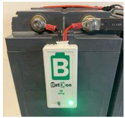
CSM module can measure charge/discharge current up 100A bi-directionally. Hall Effect current sensors can also connected to the IGU in higher current applications. In this way, the system can even measure currents of thousands of Amperes.
